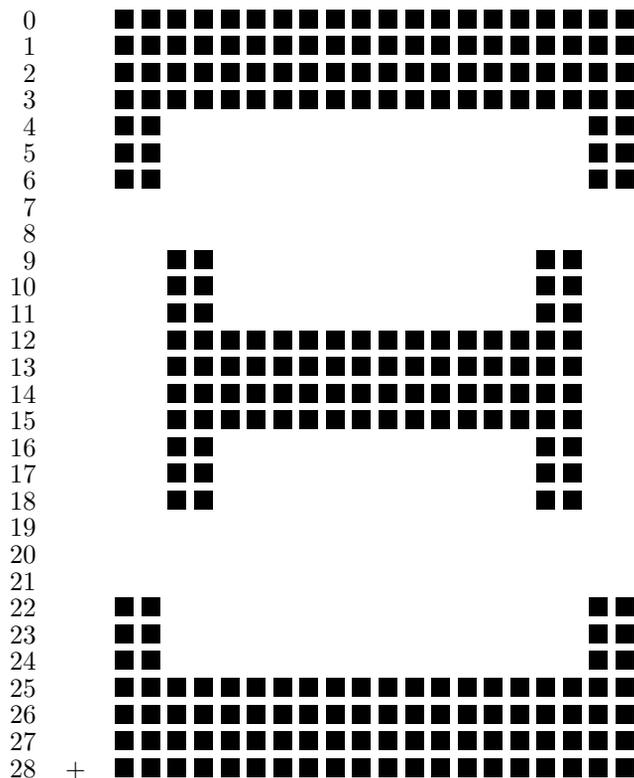
The width of the minimum bounding box for this character is 20; its height is 29. The '+' represents the reference pixel; notice how it lies outside the minimum bounding box. The *hoff* value is  $-2$ , and the *voff* is 28.
